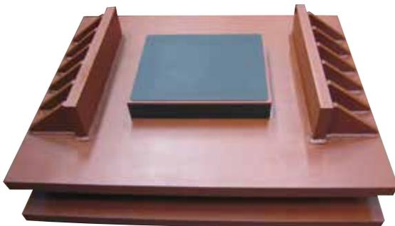
Typical assembly consists of a Lower Plate with reinforced Fluorinoid® PTFE FL129 which can be either surface mounted or recessed for high bearing pressure. The top plate is either Fluorinoid® FL129 or polished Stainless Steel.
